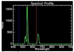
Figure 6: Emission spectrum of upconverting NPs.
