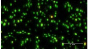
Figure 3: 50nm AuNPs on a glass slide.
