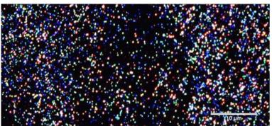
Figure 1: 30nm AgNPs Aggregating in DI Water
